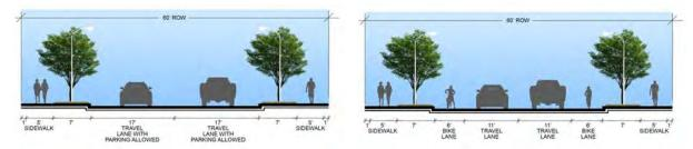
Collector streets should be sufficiently wide to allow for one lane of traffic in each direction and either curbside parking or bike lanes (typically not both), suitable to the needs of the neighborhood and the transportation network. At intersections, the corners should be provided with bulb-outs where feasible, and except where bike lanes are provided, to create the appearance of a narrower street as a traffic calming measure.
