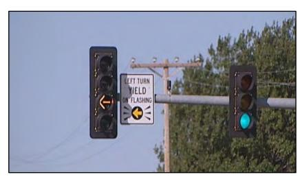
FYA signal heads have been installed on a city-wide basis
