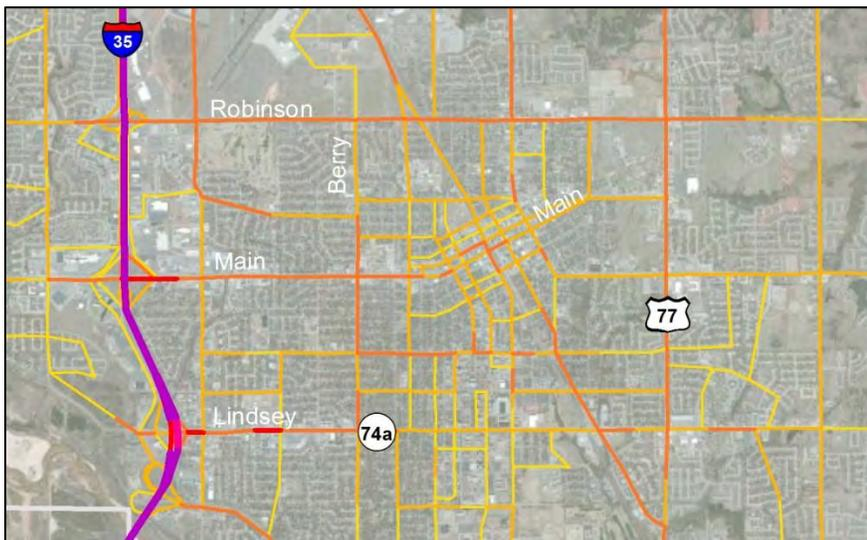
Figure 22: Norman Initial Build Scenario – AM Peak Congestion Levels
