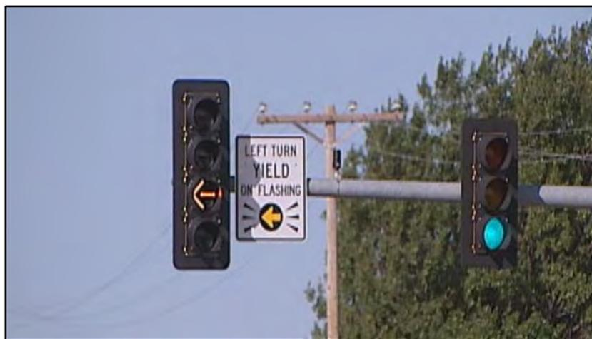
FYA signal heads have been installed on a city-wide basis
