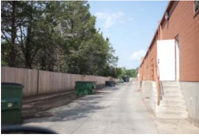
As required by City Ordinance, a six-foot stockade fence separates the backside of Alameda Square Shopping Center from adjacent houses
